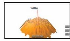
Scans below the boat -- front to back and side to side - to construct a full 3D view of the area under the boat, letting you see contour changes, fish and structure, even while stationary.
